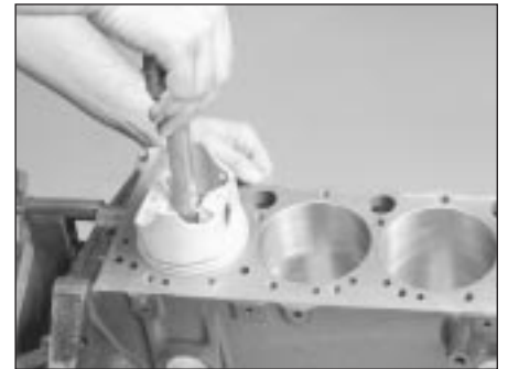
16.2 When checking piston ring end gap, the ring must be square in the cylinder bore (this is done by pushing the ring down with the top of a piston, as shown)
