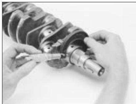
13.5 Measure the diameter of each crankshaft journal at several points, to detect taper and out-of-round conditions
