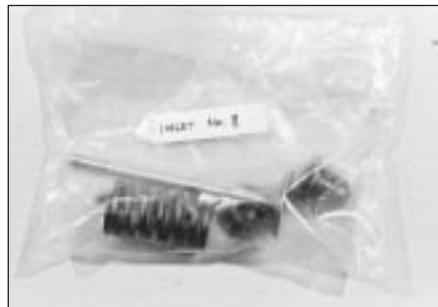
6.7 Use clearly-marked containers to identify components and to keep matched assemblies together
