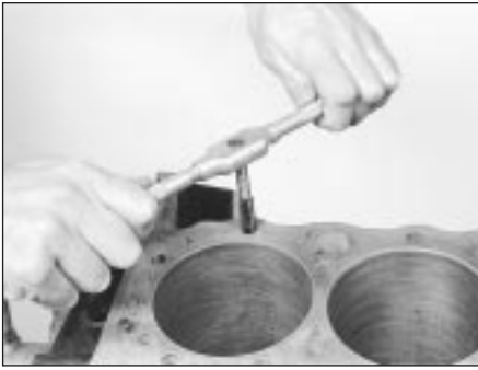
11.8 All bolt holes in the block - particularly the main bearing cap and head bolt holes - should be cleaned and restored with a tap (be sure to remove debris from the holes after this is done)
