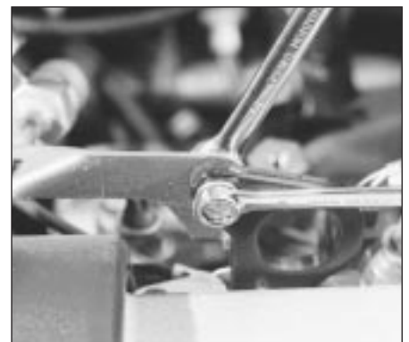
4.9B . . . unbolt the power steering high-pressure pipe . . .
