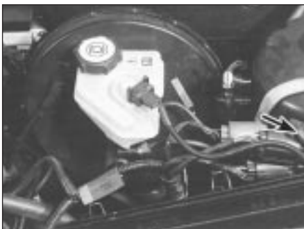
4.13A Unplug three large electrical connectors (arrowed) . . .
