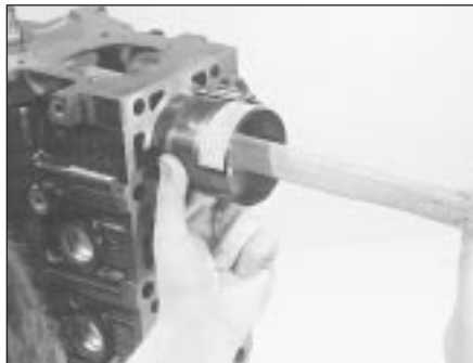
18.9 The piston can be driven gently into the cylinder bore with the end of a wooden or plastic hammer handle
