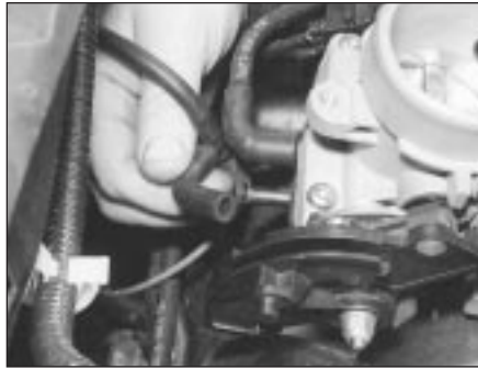
4.10A Disconnect vacuum hose shown from rear of throttle housing . . .
