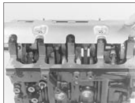
9.4 Removing the oil baffle to provide access to crankshaft and bearings
