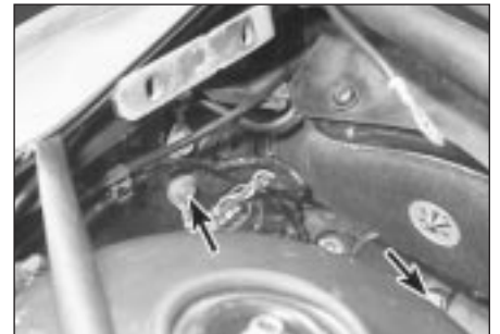
4.13C . . . and disconnect ECU wiring and earth lead (arrowed) to release engine wiring loom from vehicle body
