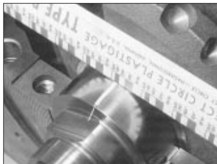
17.10 Compare the width of the crushed Plastigage to the scale on the envelope to determine the main bearing oil clearance (always take the measurement at the widest point of the Plastigage). Be sure to use the correct scale; Imperial and metric scales are included
