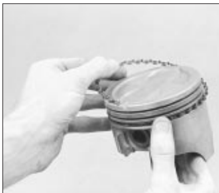
16.7B DO NOT use a piston ring installation tool when installing the oil ring side rails
