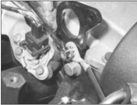
4.9C . . . and the earth lead from the cylinder head rear support plate/engine lifting eye
