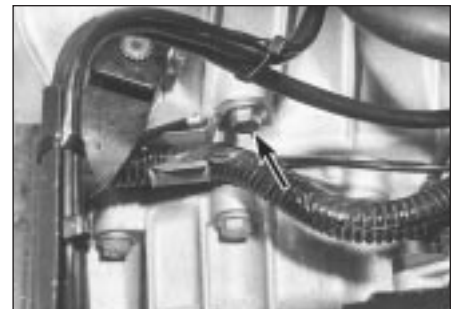
4.11 Unbolt the engine/transmission-to-body earth lead - hidden behind wiring loom guide - from location (arrowed) on the transmission's top surface
