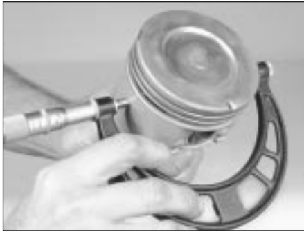
11.15 Measure the piston skirt diameter at right-angles to the gudgeon pin axis, just above the base of the skirt
