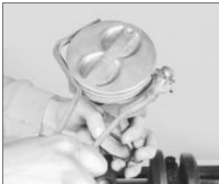
12.4A The piston ring grooves can be cleaned with a special tool, as shown here . . .
