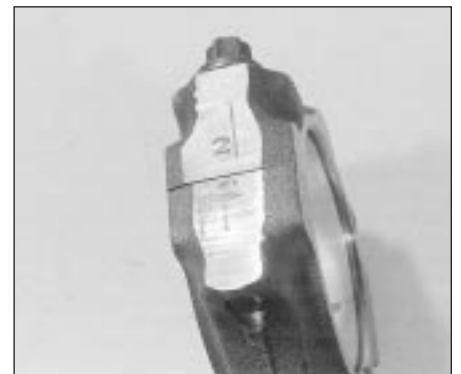
18.11 The connecting rod and big-end bearing cap of each assembly must share the same etched cylinder number, visible from the same (front/exhaust) side of the engine
