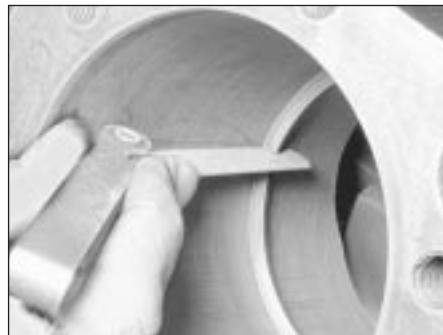
16.3 With the ring square in the bore, measure the end gap with a feeler gauge
