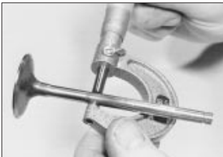
7.12 Measuring the diameter of a valve stem - if any significant difference is found in the readings obtained, excessive valve stem wear is indicated
