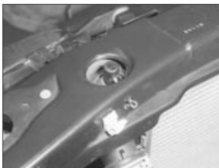
4.25A Use split pins as shown to secure radiator in its raised position . . .
