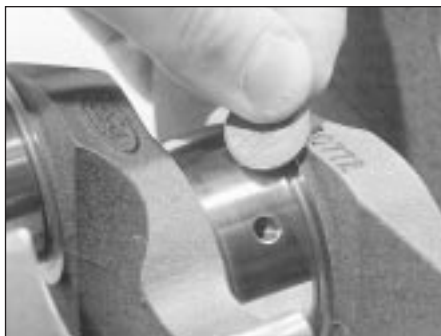
13.3 Rubbing a penny lengthwise along each journal will reveal its condition - if copper rubs off and is embedded in the crankshaft, the journals should be reground
