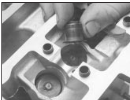
8.3 Valve spring pressure is sufficient to seat lower seat/stem oil seals on reassembly
