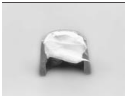
8.5 Apply a small dab of grease to each collet before installation - it will hold them in place on the valve stem until the spring is released
