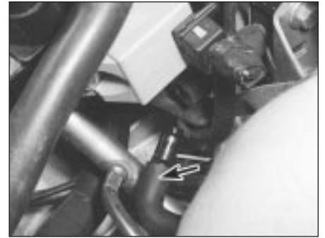
4.10B . . . vacuum hose (arrowed) from union on left-hand end on inlet manifold . . .
