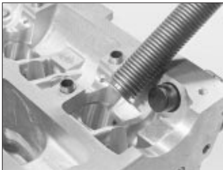
6.6B . . . can be replaced by home-made tool if suitable spring can be found
