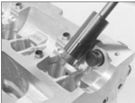
6.6A Ford service tool in use to remove valve spring lower seat/stem oil seals . . .
