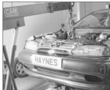
4.35 Lowering the engine/transmission unit out of the vehicle
