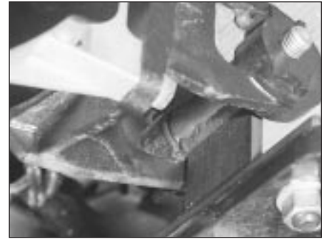
4.49 Special tool required to hold engine/transmission unit precisely, so that mountings can be tightened into correct position
