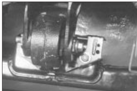
4.50D . . . then refit front mounting - do not forget wiring connector bracket - tighten the mounting's nuts first, then its centre bolt
