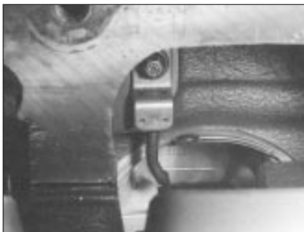
11.1F . . . but note that piston-cooling oil jets (where fitted) must be renewed as a matter of course whenever engine is overhauled
