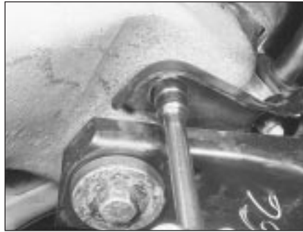
4.47B . . . but alternative methods using ordinary hand tools can achieve acceptable alignment, with care
