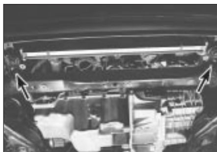
4.25B . . . while you unbolt the bottom mountings (arrowed) - note that the mountings are handed, and do not lose the mounting rubbers
