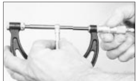
11.14C The gauge is then measured with a micrometer to determine the bore size
