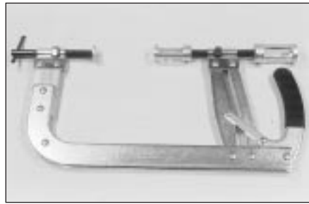
6.3B . . . or purpose-built special version, is required to compress valve springs without damaging cylinder head . . .
